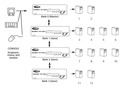
The OmniView<sup>™</sup> SE has the capability to be daisy-chained to additional units for control over more computers. Up to four OmniView<sup>™</sup> SE units can be daisy chained together, whether 2-Port, 4-Port, or a mixture of both. The example above shows two OmniView<sup>™</sup> SE 2-Port units and two OmniView<sup>™</sup> SE 4-Port units daisy-chained together.
